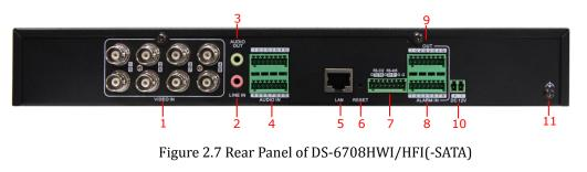
*Note:* DS-6701/6704 HWI-SATA and DS-6701/6704 HFI-SATA models provide 1/4 video input and 1/4 audio input interfaces on the rear panel.
