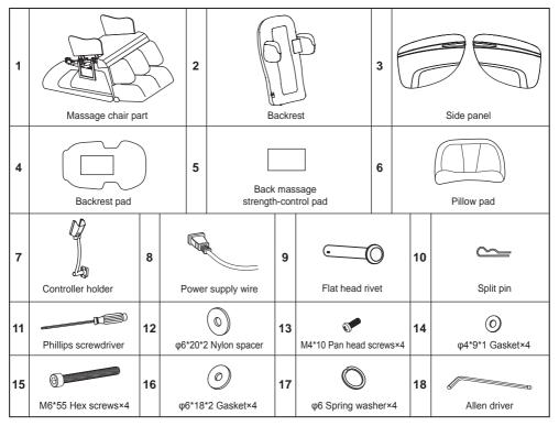
Step 1: Remove the chair parts out of the two cartons:
