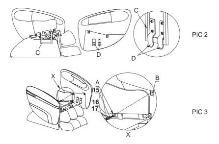
Step 4: Repeat step 2 and step 3 to install the other side panel.
