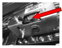
The locking system is provided with an unlocking lever
