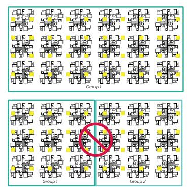
When configuring open plan offices with SpaceWise DT, large groups of 30-40 luminaires are recommended to maintain the lighting aesthetics of the space. Smaller groups may turn off more frequently than desired.
