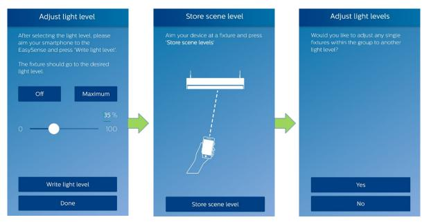
For a given scene, individual fixtures within the group can be configured to different light level settings. This is beneficial for example in a conference room where fixtures closer to the projection wall are desired to be dimmed/off while other fixtures in the same group are desired to be at higher light levels on the same scene.
