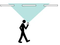
For proper commissioning, hold the phone above your head, pointed at the luminaire that you wish to target. This will help ensure that the IR range or cone is restricted to just one luminaire, and only that luminaire will react. Holding the phone closer to eye level or lower will result in a wider IR range or cone. This will cause multiple luminaires to receive the signal.
