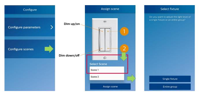
The scenes are selectable via the scene buttons of the switches associated either to fixture or an entire group. In any case, the configuration proceeds through the "Adjust light level" screen that enables the user to select desired light level for the selected scene.
