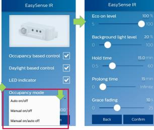
Once all parameters have been set, select confirm & either save these parameters as a profile for future reference as per the instructions in section 5e or users can skip the saving profile option and push these settings on a single fixture or the entire group.
