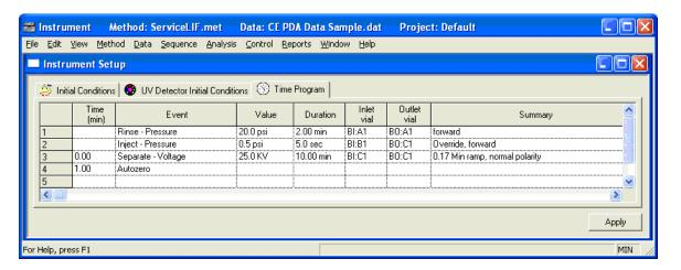
The rinse and separation vials contain borate and the inject vial contains a 1:1 mixture of fluorescein and buffer. A peak is detected at about 5 minutes. Optimize the integration so only the main peak and small contaminant peaks are detected. Annotate the peak with S/N (ASTM). On a calibrated instrument, the S/N (signal-to-noise ratio) should be greater than 10,000.
