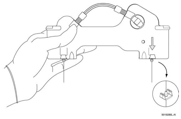
2 Inspect the seals. If they appear worn, damaged, or leaking, replace with new seals.
