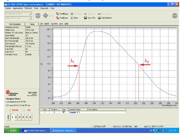
Figure B.2 Example of Calculating Center Wavelength using Full Width at Half Maximum
