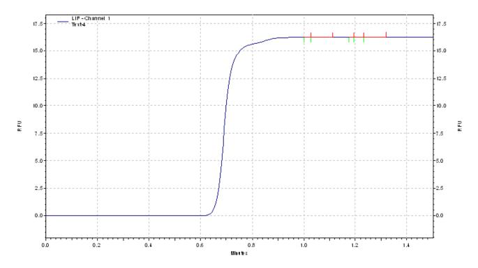
(Water and fluorescein in 30cm 50 µm BFS capillary.)
