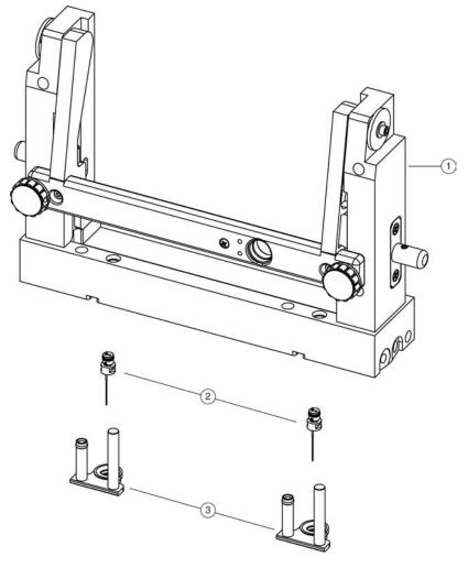
Figure 2.1 Interface Block, Electrodes, and Opening Levers
