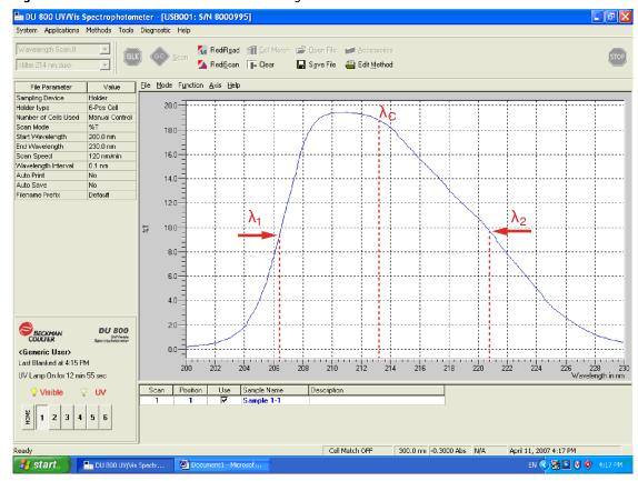
Figure B.3 Calculated Result of Center Wavelength
