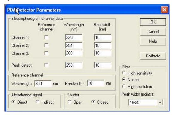
4 Select **Calibrate** to start the calibration sequence. The calibration requires approximately two minutes. Do not try to access the instrument during the calibration process.
