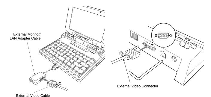
Figure 34. Connecting External Video to System
