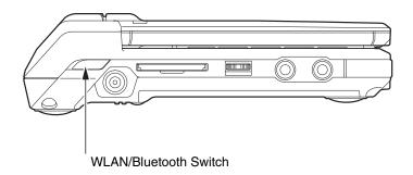
Figure 41. Wireless LAN/Bluetooth On/Off Switch Location
