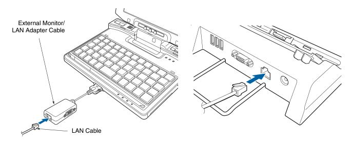
Figure 36. Connecting the LAN and Adapter
