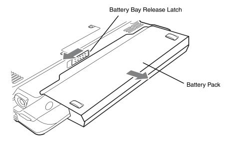
Figure 28. Removing a Battery
