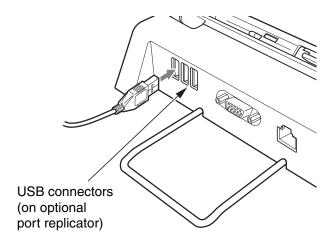
Figure 33. Connecting USB to Port Replicator
