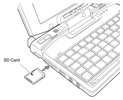
Figure 29. Installing a Secure Digital Card
