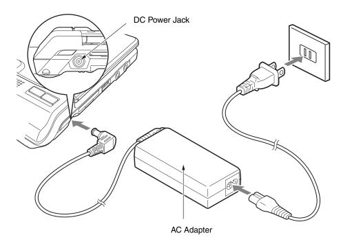
Figure 27. Connecting the AC Adapter
