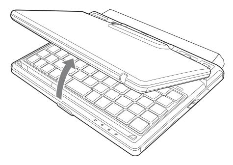
Figure 8. Opening the Display Panel
