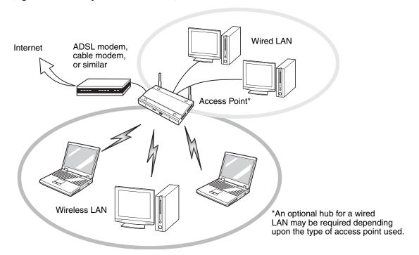
Figure 40. Access Point (Infrastructure) Mode Network
