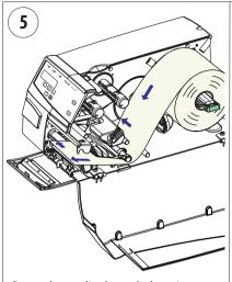
Route the media through the print mechanism. Then push it inwards as far as it will go. Close the edge guide on the media supply post.
