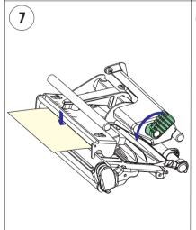
Turn the printhead lift lever counterclockwise to engage the printhead.
