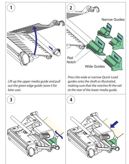
If necessary, adjust the outer Quick-
