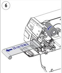
Route the ribbon through the print mechanism and pull out approximately 20 cm (8 inches) of ribbon.
