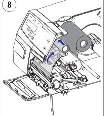
Slide the empty cardboard core onto the ribbon rewind hub so the ribbon is wound up when the hub rotates counterclockwise.
