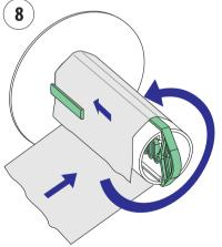
Insert the start of the liner under the lip of the takeup hub, then rotate the hub counterclockwise a few turns to wind up some of the liner.
