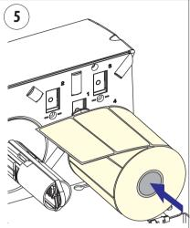
Fit a new roll of labels on the supply post.
