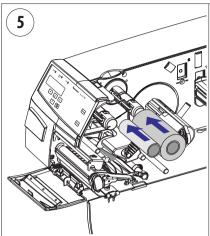
Slide the ribbon roll onto the supply hub so the ink-coated side faces down when the ribbon is routed through the print mechanism.
