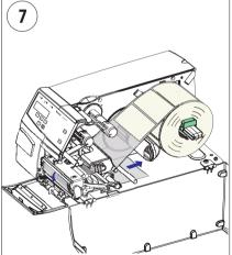
Close the edge guide. Route the liner around the tear bar and the liner drive roller and back under the print mechanism and guide shaft.
