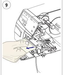
Pull out the cleaning card. If necessary, repeat the process with a fresh cleaning card.
