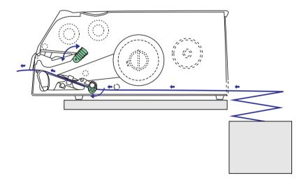
This diagram shows the media path from an external supply. In case of the standard edge guide (as opposed to Quick-Load guides), turn it to vertical position.
