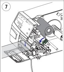
Without releasing the ribbon, turn the printhead lift lever counterclockwise to engage the printhead and lock the ribbon.
