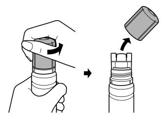
**Caution:** Do not shake or squeeze the bottle. Do not touch the top of the bottle after removing its cap.
