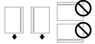
To load a sheet of paper longer than legal size, close the paper support and flatten the leading edge of the paper as shown.
