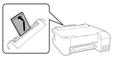
2. Pull out the output tray and open the paper stopper.
