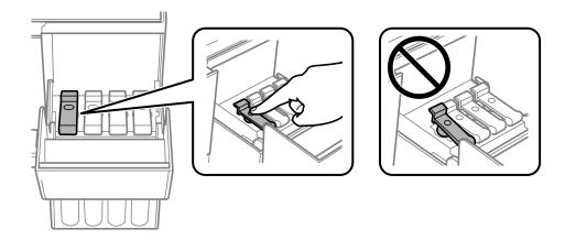
**Note:** If any ink remains in the bottle, replace the bottle cap and tighten it. Store the bottle upright for later use.
