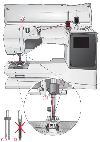
Note: Only use symmetrical twin needles (C). Do not use this type of twin needle (D), since it may damage your sewing machine.
