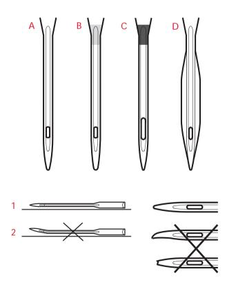
Note: Change the needle often. Always use a straight needle with a sharp point (1). A damaged needle (2) can cause skipped stitches, breakage of needles or snapping of thread. A damaged needle can also damage the stitch plate.
