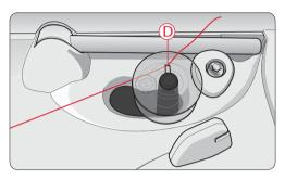
Note: When using an earlier version of HUSQVARNA VIKING® bobbins that do not have a hole, wind several turns of thread on the bobbin to get started.
