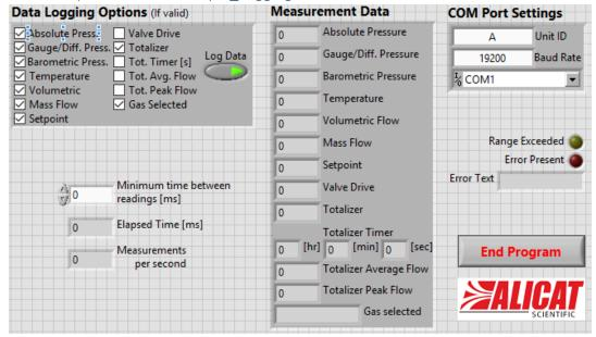
This version of the simplified drivers is the same as the "Simplified Driver Example," except for the fact that it has an added segment of code that logs the desired data into a file each time the data is received.
