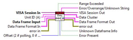
Parses data string obtained from an Alicat device according to data flag inputs, and if none are present the device will query the data flags (adding a considerable amount of time to the VI's execution). Outputs cluster of data, retrieved/used data flags, and error/overrange/unknown indicators and strings.
