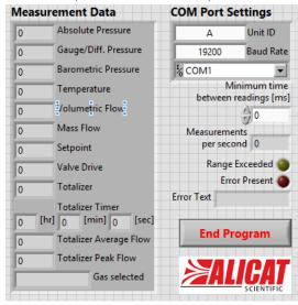
This is a simplified version of an example program that only contains the measurement data that is read out from an Alicat device. By adjusting the minimum time between readings, a delay between successive reads can be added (utilizing the LabVIEW "Wait" sub-VI; if the minimum time is set to a value lower than the lowest value achievable with the current settings (limited by the data rate and the number of characters sent in each data frame), this will have no effect.
