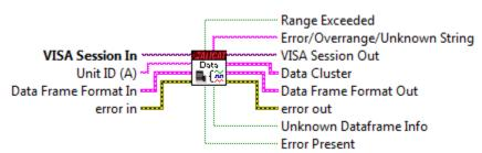
Polls the Alicat device for its data frame and outputs cluster of data, retrieved/used data flags, and error/overrange/unknown indicators and strings. Data is parsed according to data flag inputs, and if none are present the device will query the data flags (adding a considerable amount of time to the VI's execution).
