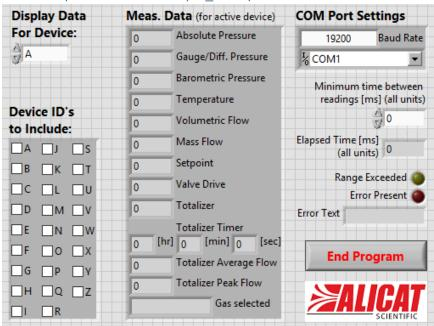
This version of the simplified drivers is the same as the "Simplified Driver Example," except for the fact that it has an added segment of code that initializes and queries all selected devices. The data displayed can be selected to be associated with any of the connected Alicat devices by using the "Display data for device:" control. This example shows one easy way to read data from multiple Alicats in quick succession using a for loop that is auto-indexed on an array of device identifiers.
