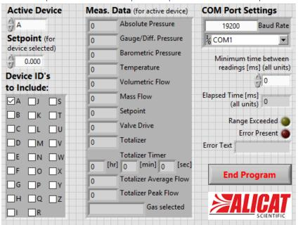
This version of the simplified drivers is the same as the "Simplified Driver Example\_Multiple Devices," except for the fact that it has an added segment of code that writes a setpoint to the specified device (if the setpoint has changed).
