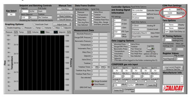
To connect to an Alicat, simply select the appropriate COM port that the Alicat is connected to and ensure that the Unit ID and Baud rate controls are set to match the values on the Alicat that you would like to talk to. The example VI will continually try opening the COM port and querying for a connected Alicat; if no Alicat is connected that matches these settings, the program will close the COM port, wait for a given amount of time and retry.
