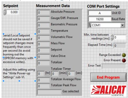
This version of the simplified drivers is the same as the "Simplified Driver Example," except for the fact that it has an added segment of code that writes a setpoint to the specified device (if the setpoint has changed).
