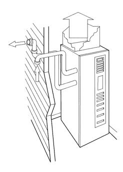
• Keep the area around your furnace clear and free of combustible materials, gasoline, and other flammable liquids and vapors.
