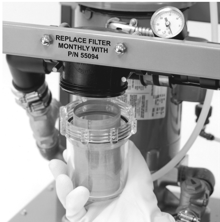
Figure 12. Intake Solids Collector Location
