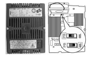
**NE143P charger:** On the front next to the connections, a contactor lets you select the battery type: GEL for a gel type / PB for a lead type.
