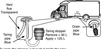
To apply the stopper, just push it inside the pipe. To remove the stopper.
