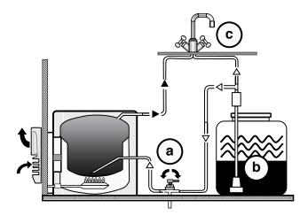
position) until the water heater is full of water, all air has escaped and water is running freely.
