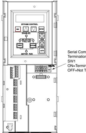
Serial Communications Termination Resistors SW1 ON=Terminated OFF=Not Terminated
