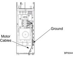
Motor Connections – Standard E-Clipse Bypass Configurations (Wall Mounted)
