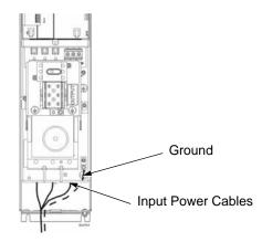
Connect input power to the terminals of the disconnect switch or circuit breaker. Connect the equipment grounding conductor to the ground lug at the top of the enclosure. The figure below shows the connection points for Standard E-Clipse Bypass configurations. Also see "Connection Diagrams – Standard E-Clipse Bypass" on pages 10 and 11.
