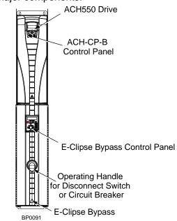
The following shows the front view of the ACH550 E-Clipse Bypass vertical configuration, and identifies the major components.
