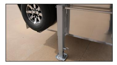
Fig.14 Drop-leg Jack Arrangement
