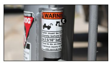
Fig.5 Gooseneck Safety Warning Labels (Bottom of Coupler)
