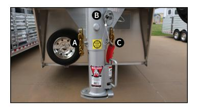
Fig.13 Gooseneck Ball Receiver and Height Adjustment
