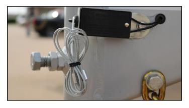
Fig.11 Breakaway Brake Cable Lanyard
