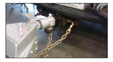
Fig.10 Safety Chain Arrangement
