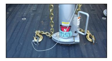
Fig.16 Safety Chain Arrangement
