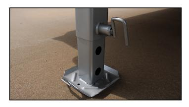
Fig.15 Drop-leg Mechanism
