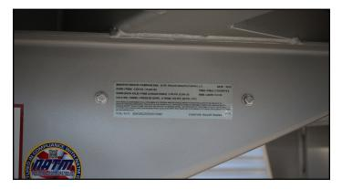
Fig.8 Gooseneck Trailer VIN Certification Label
