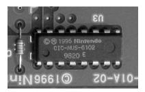
Each cartridge contains a small microcontroller (CIC) that maintains constant communication with a similar chip (PIF) inside the N64 console. If the chip is absent, the wrong type, or does not exactly match the region, the system will not boot.
