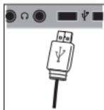
Plug the large end of the USB cable into a USB port on the PC.
