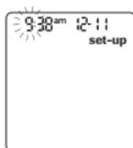
Press and **hold**
