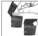
Remove a test strip from the test strip container.
