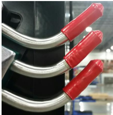
Figure 6 PRD vent tube caps must be in place. If vent caps are missing, inspect the vent tubes for moisture and debris, and replace the caps.
