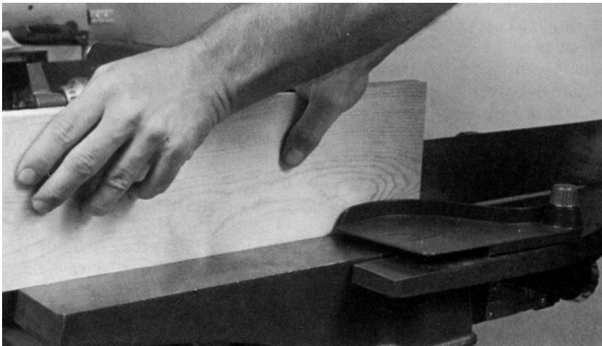
Figure 6-5. (A) Begin the cut using your left hand to steady the stock and your right hand to feed it forward. (B) As the stock nears the halfway point, reposition your left and to the outfeed side of the jointer. (C) Continue to steady the stock with your left hand while you move your right hand to the outfeed table. Finish the cut by pushing the end of the stock past the cutterhead with both hands.
