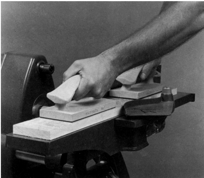
Figure 6-12. A push block will help maintain even pressure, give better control over the stock, and keep your hands out of the danger zone.
