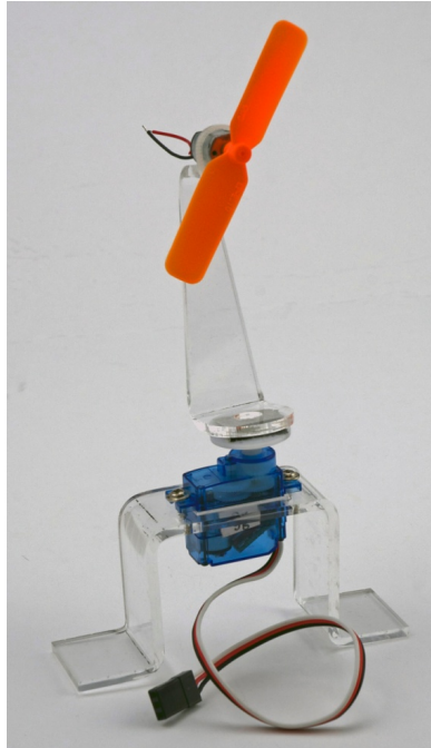
Figure 5: Reference design for the structure, and list of components for the desktop fan. The Arduino Inventor's Kit contained all components except for the propeller and the acrylic used for structural support.
