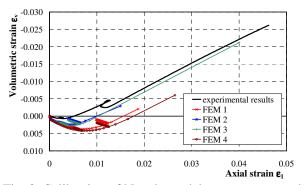
Fig. 8. Calibration of Nova's model parameters, graph  $\epsilon_1$  -  $\epsilon_v$
