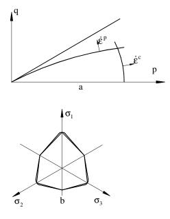
Fig. 5. Volumetric yield surface (a) and deviatoric yield surface (b) for Vermeer's model
