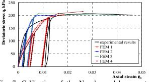
Fig. 7. Calibration of the Nova's model parameters, graph  $\varepsilon_1 - q$
