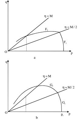
Fig. 4. Yield surface (a) and plastic potential (b) for Nova's criterion
