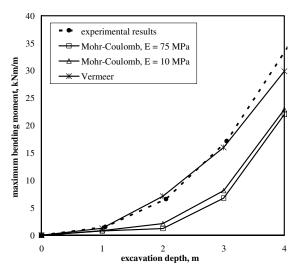
Fig. 15. Maximum bending moments in the retaining wall
