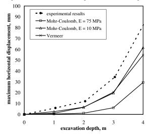
Fig. 13. Maximum horizontal displacements of the retaining wall
