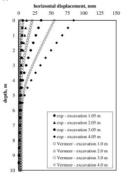
Fig. 14. Horizontal displacements of the retaining wall
