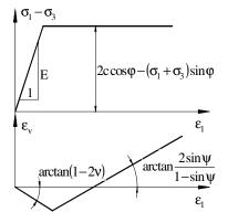
Fig. 2. Axial symmetric triaxial compression test modeled using Mohr – Coulomb criterion
