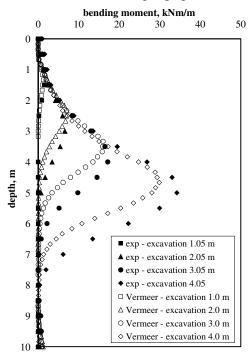
Fig. 16. Bending moments in the retaining wall
