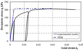
Fig. 6. Calibration of the Mohr-Coulomb parameters
