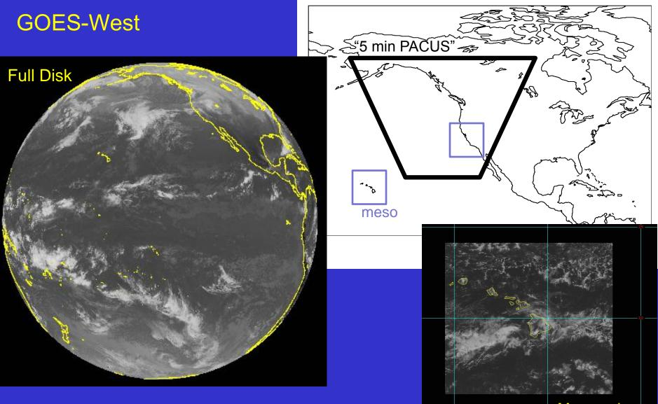
Possible scan modes for the west ABI (per hour):MesoscaleContinuous FD--Full disk scan every 5 minutes, ORFLEX--Full disk scan every 15 mins + continuous 5-min "PACUS" images + twoselectable Mesoscale areas with continuous 1-min scans, OR...
