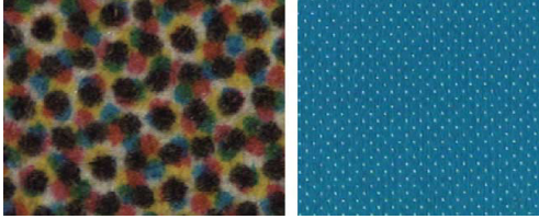
Fig. 1. Left: An enlarged view of a part of a newspaper picture that was created by printing dots of cyan, magenta, yellow and black inks. Right: An example of an image containing very small areas of one colour and large areas of other colour.
