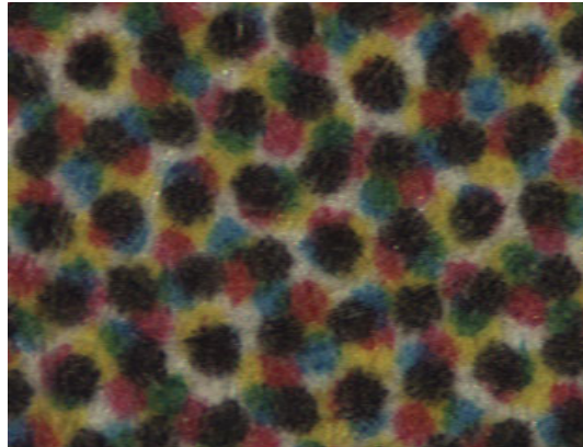
Fig. 1. An enlarged view of a part of a newspaper picture that was created by printing dots of cyan, magenta, yellow and black inks.
