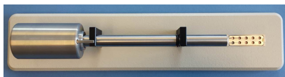
Figure 2. Fischione Instruments' Grid Specimen Holder (part number 011-0002).
