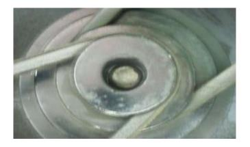
Better know as 'idler wheels' are used to alter the rpm of the final drive. By placing an idler wheel in between the motor pulley and final drive we can reduce or increase the drive speed. Idler wheels are not powered in themselves, they simply transfer drive via the vee belt. The spindle for the idler wheel will need to run freely in bearings.
