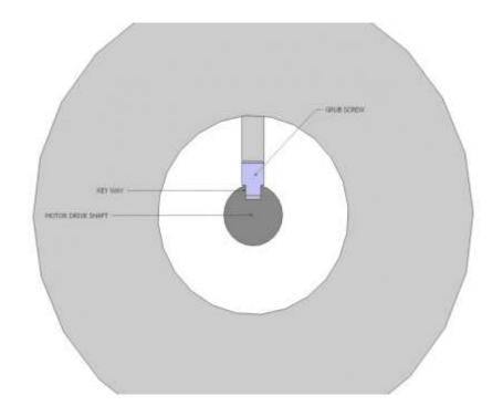
If there is nowhere obvious on the pulley to drill and tap a grub screw, you can drill into the bottom of one of the grooves as shown below, however, you must ensure you have removed any sharp edged afterwards and that the grub screw is well below the surface so as not to interfere with the vee belt.
