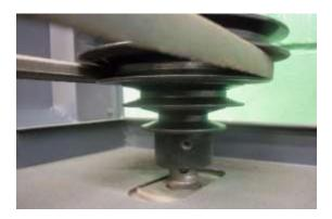
Not all vee pulleys are secured with a key and keyway. In the image above, the pulley attached to the motor of this pillar drill is secured to the drive shaft using what is known as a 'grub screw' or 'socket screw'.
