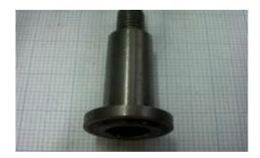
You will need to machine a 'sleeve' that will fit over the small motor shaft and increase its' diameter. You will also need to ensure that the sleeve can fit securely to the motor shaft and that the pulley can then fit securely to the sleeve. All of this will have to be done very accurately.
