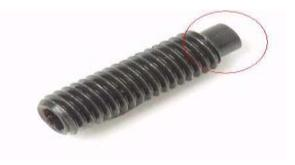
These are small screws that are tightened with a 'hex key' better known as an 'allen key'. It's important to make sure that the grub screw is fastened into the keyway of the motor shaft and not onto the shaft itself, otherwise the pulley will come loose and the motor shaft will get damaged.
