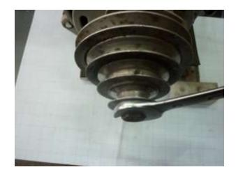
Finally, a nut and washer add extra security to prevent the pulley coming off.
