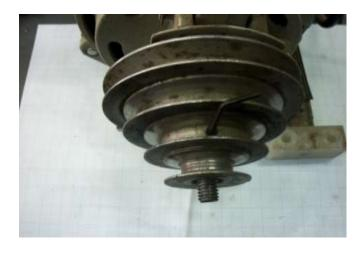
Above you can see how the pulley can now be fixed to the sleeve buy using a grub screw into the 'D' dent.
