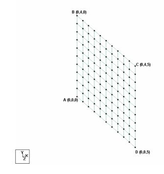
Here X coordinate is 0; therefore the plane is Y-Z, a good setup for a wall.
