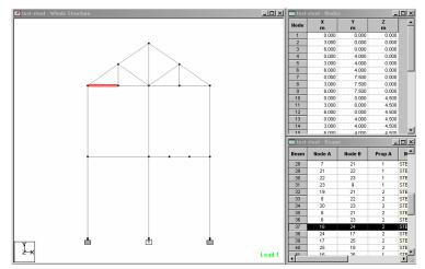
Multiple Selection • Select the first Node, Beam, or Plate, then hold down the Ctrl key at the keyboard, and click other Nodes, Beams, and Plates. Check the figure below.
