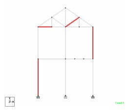
• From the Data Area, click on the number of the Node, Beam, or Plate, it will be highlighted. Then hold the **Ctrl** key at the keyboard, and click on other numbers; it will be highlighted as well. Check the figure below.
