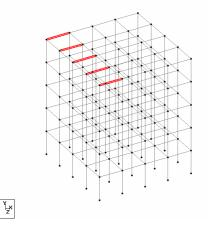
Note ■ To speed up the selection method of 3D geometry, use Window, which will enable the user to select multiple Nodes, Beams, and Plates, in the 2D View.
