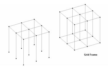
**Frame Models /** Floor Grid is two-dimensional structure is the X-Z plane only. Floor Grid The purpose is to create a mesh of beams in the X and Z direction
