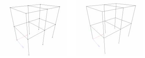
From the toolbars, click XY View (Elevation), or select View/ Elevation (XY) View. This will show 2D view, to see XY plane of the structure. See the illustration below (this is a structure of X=6m, Y=15m, Z=12m and shown as Perspective, and will be shown in all illustration below):
