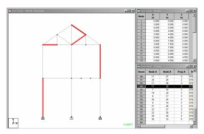
• Make a Window around the needed Nodes; Beams, or Plates, by clicking in an empty place of the STAAD Pro window, and holding down the left button, moving to the other corner and releasing the button, what ever inside the Window will be selected automatically. Check the figure below:
