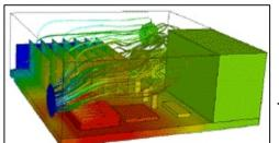
Evaluation of cooling air flow behavior inside a computer system chassis
