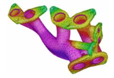
Postprocessing: Finite Element Analysis and Computational Fluid Dynamics results visualization
