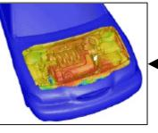
Simulation of underhood thermal cooling for decrease in engine space and increase in cabin space and comfort
