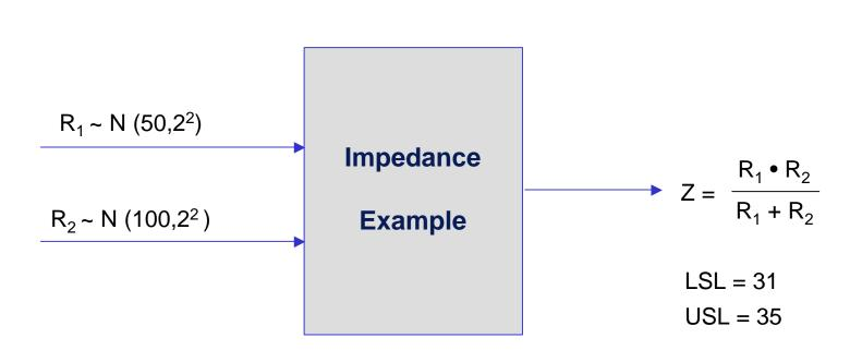
If we were able to change a resistor's standard deviation, which resistor,  $R_1$  or  $R_2$ , would have the greater impact on the dpm of Z (impedance)?
