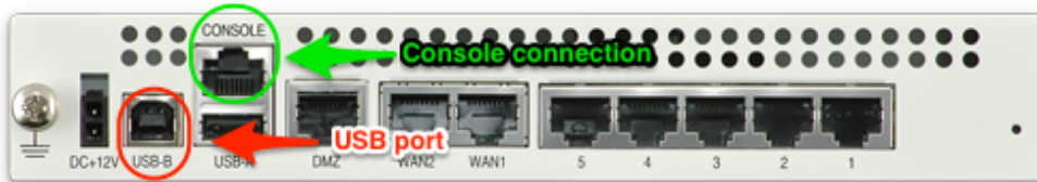
FortiGate 60C with RJ-45 Console port
