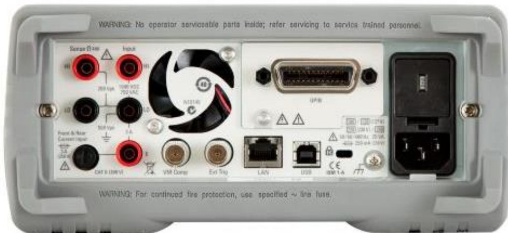
Figure 12. Back end of a typical instrument, showing signal connections (left), I/O to the PC (middle), and AC power (right)
