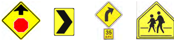
Stop Sign Ahead Sharp Curve Ahead Advisory Speed Around Curve School Crossing
