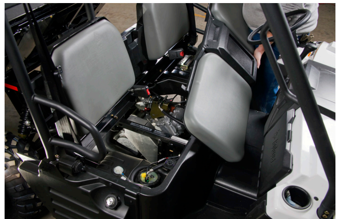
Liquid-cooled engine with radiator under the seat.
