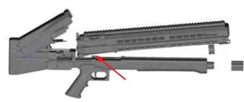
Press down firmly to make sure the barrel is fully mounted into the receiver then replace the barrel retaining cap making sure it is screwed down snuggly. Close the upper stock, slide the action into the forward and locked position, then close the ejection port door.
