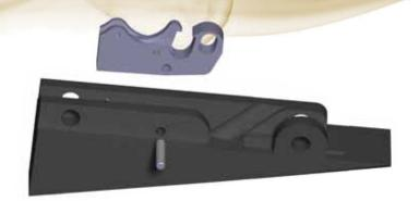
The sear / secondary sear assembly can be removed from the gearbox housing by pushing out the sear pivot pin (33)
