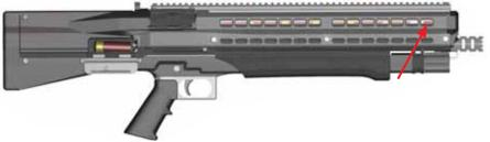
Now with both magazines fully charged and the action in the full rear position the 15<sup>th</sup> shell can be placed directly in the chamber of the barrel (12).
