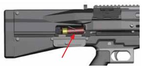
The action will automatically release when the shell is fired; the action should then be moved fully rearward in a positive manner to expend the spent cartridge and have a new live round loaded onto the shell loading ramp (15).
