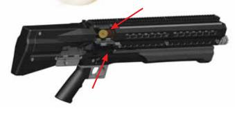
which will hold the magazine follower in the magazine tube, leaving the monobloc port open to receive shells (9).
