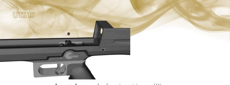
Lower stock - remove the safety spring retaining screw (41)
