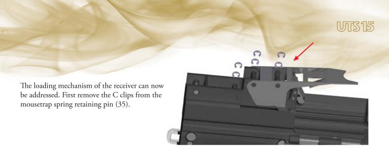
With the receiver held in a vice or similar holding fixture, hold the mousetrap spring down by placing a block of wood or similar material on the spring coils while the mousetrap spring retaining pin is removed with a drift punch. Remove the C clips from the mousetrap spoon pivot and forward pin (36) and remove pins from assembly.
