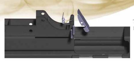
The mousetrap trigger plate and spring is held in place with a headless screw, with a similar spring bearing screw directly below (37).
