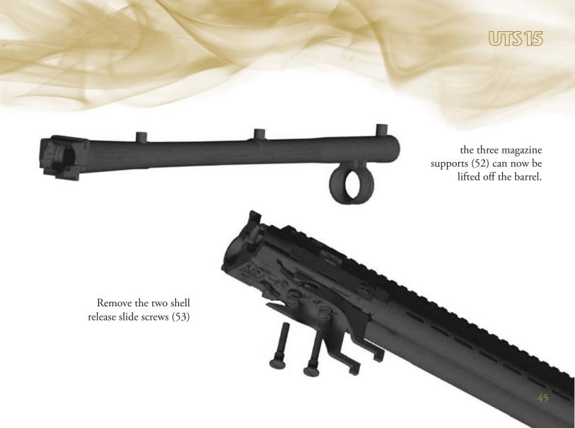
with their washers and tensions springs and lift off the shell release slide (54).
