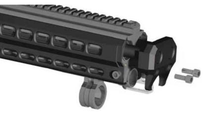
**Barrel / magazine assembly** - Remove the magazine cap (46) by unscrewing the two forward caps screws
