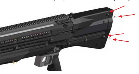
**Receiver** – remove C clips from the receiver retaining pins and upper stock hinge pin (26).
