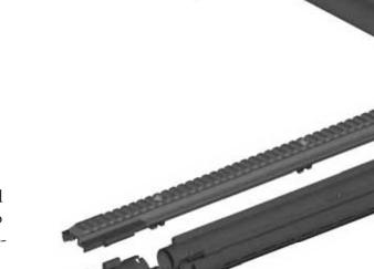
This will also free the top rail from the monobloc and allow the magazine tubes to be removed from the monobloc as well (55 A).
