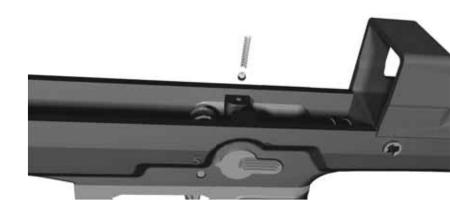
from the stock and drop out the safety spring and plunger (42).
