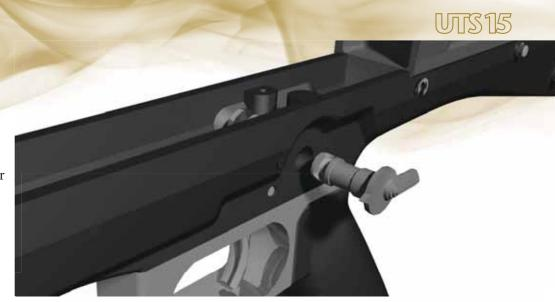
Rotate the safety a little over 90° until the machined clearance flat on the safety is over the trigger bar and slide safety out of the stock(43)
