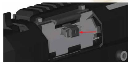
The shell follower should then be pushed forward with the end of you thumb until it passes the magazine shell catch (8)
