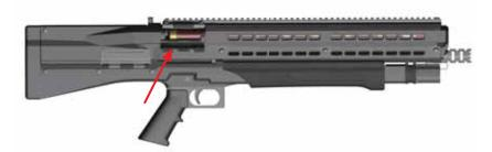
When the loading port door is closed the shells held in the magazine tube will be released, charging the full seven 2 ¾" or six 3" shells into the ready to load position, with an audible sound of the shells moving rearward to the rear of the monobloc.
