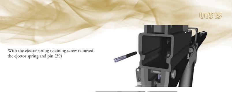
may fall free or can be pushed out of the receiver with a thin screw driver or wire. Carefully drive the ejection port door retaining pin (40) out of the receiver being conscious of the ejection port door spring; this completes the disassembly of the receiver.
