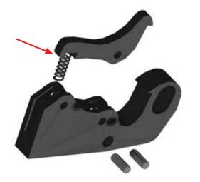
with a drift punch. The secondary sear can then be removed by driving out the secondary sear pivot pin (34)
