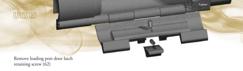
being conscious of the loading port door latch spring underneath. Unscrew the interrupter retaining screw (63) from the monoblock
