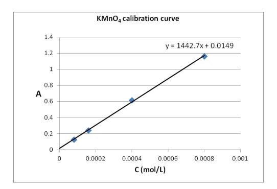
On the graph you can see that the trend line does not pass exactly through zero. This is as expected: it may be due to the statistics of the data point, which are not exactly on the straight line due to random errors in the concentration and/or the absorbance reading, or to the fact that there is a remaining solution absorbance (relative to the blank) for the standards. For these reasons, you should not choose the "set intercept" box when formatting the trendline.
