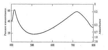
Figure 1: The absorption spectrum of the Fe<sup>3+</sup>-salicylate complex.
