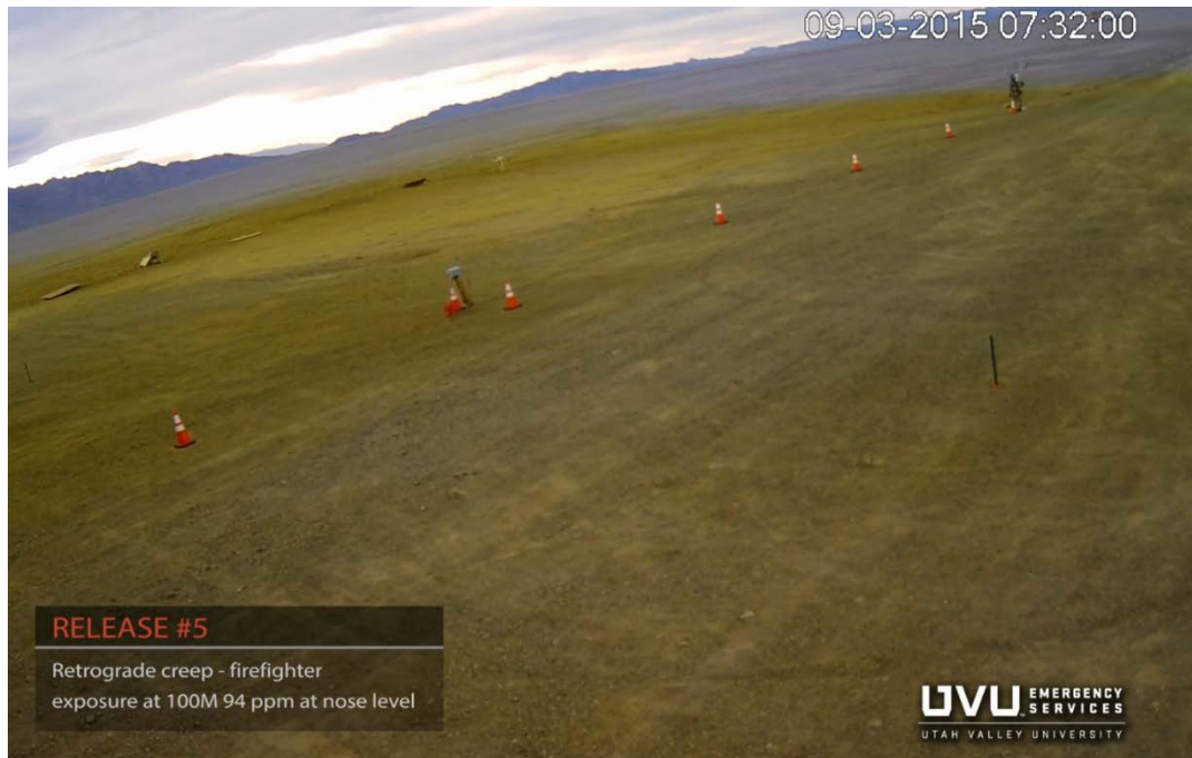
Figure 11. Release 5, 2015. Retrograde creep of the visible plume against a 2.7 m/sec wind. The firefighter mannequin is 100m upwind as seen in the upper right corner.
