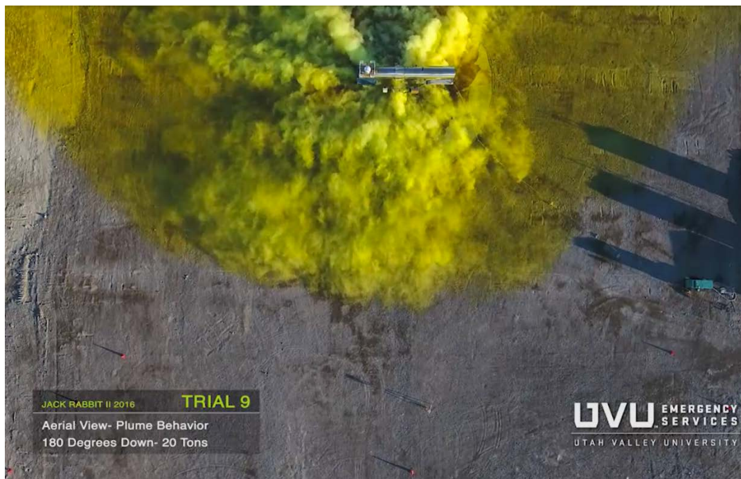
Figure 12. Release 9, 2016. The small cone in the extreme bottom center of the screenshot is 50m upwind during this 20 ton release with a wind speed of 3.55 m/sec.
