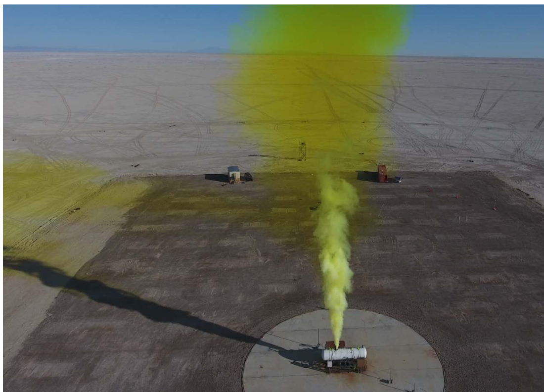
Figure 37. Release 8, 2016. The vertical plume and the subsequent ground shadow was somewhat unanticipated and, coupled with ground video, provided a 3-D type of visual effect. Concentrations inside the vehicles were surprisingly low as the chlorine landed on the pad downwind.
