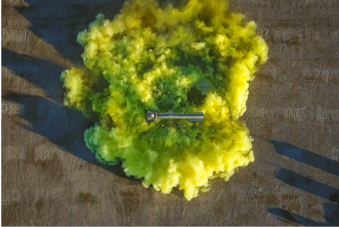
Figure 38. Release 9, 2016, 20 tons. Seconds after the release. The UAV provided upwind and downwind angles of the largest of the plumes and depicted the best view of the release behavior found in no other video. Compare with Figure 39.
