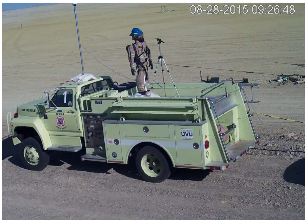
Figure 18. Release 2, 2015. Firefighter mannequin on top of an engine simulating an escape from a plume. Visible plume in the background. 49.9 ppm at the nose level, 100 m downwind.
