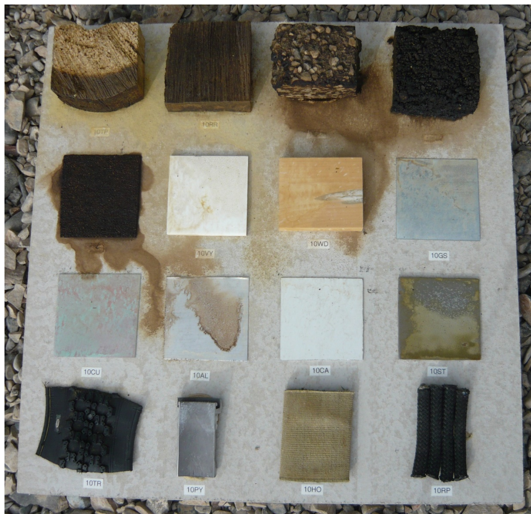
Figure 49. Release 5, 2015. Witness board #10 after complete evaporation of the liquid chlorine exposure. Note the dissolving hydrocarbons and metal corrosion.
