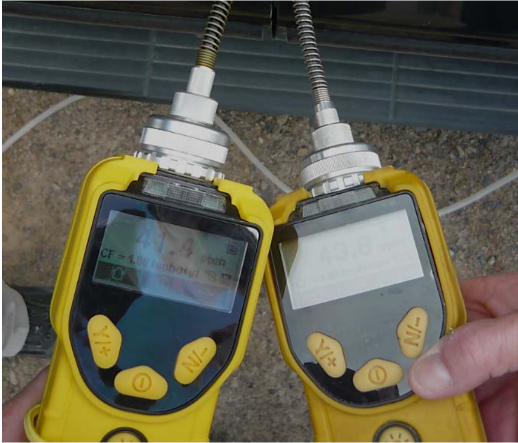
Figure 32. PID side by side comparison. The left PID (UVU #12) was exposed multiple times to high concentrations and then recalibrated and challenged by a new, never exposed PID on the right. Left PID reads 41.4 ppm, right PID reads 43.8 ppm (glare).
