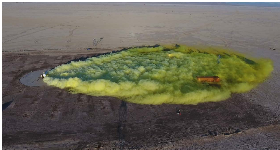
Figure 36. Release 7, 2016. 135° downward angle and high wind speeds contributed to a spectacular visual of the plume's energetic activity and its behavior when encountering the structures on the grid.
