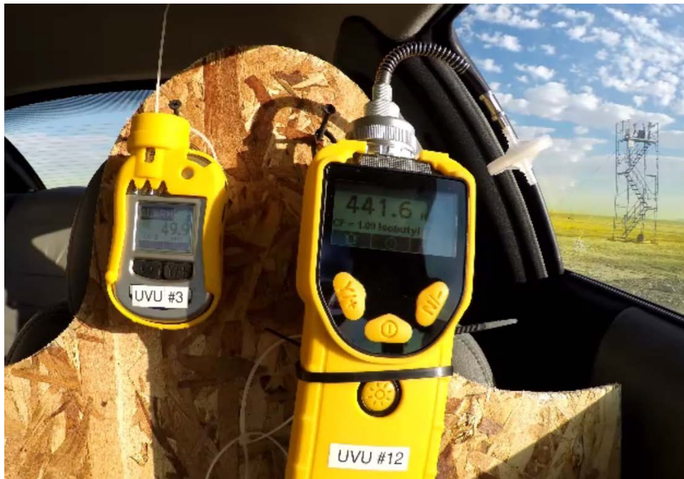
Figure 31. Release 7, 2016. A camera captures the maximum concentration inside vehicle #1 at 441.6 ppm on the PID and 49.9 ppm locked on the electrochemical sensor. Visible chlorine cloud outside.
