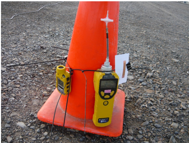
Figure 13. Release 9, 2016. A UVU ToxiRAE® and a DPG MiniRAE® detector at the 50m cone upwind.
