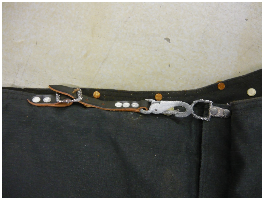
Figure 46. Release 5, 2015. Corroded metal parts on turnout pants exposed to ~24% chlorine concentration.
