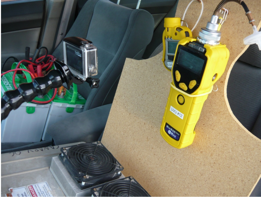
Figure 15. A typical vehicle co-location set up with ToxiRAE®, MiniRAE® PID (11.7) and UV Canary and capture camera.
