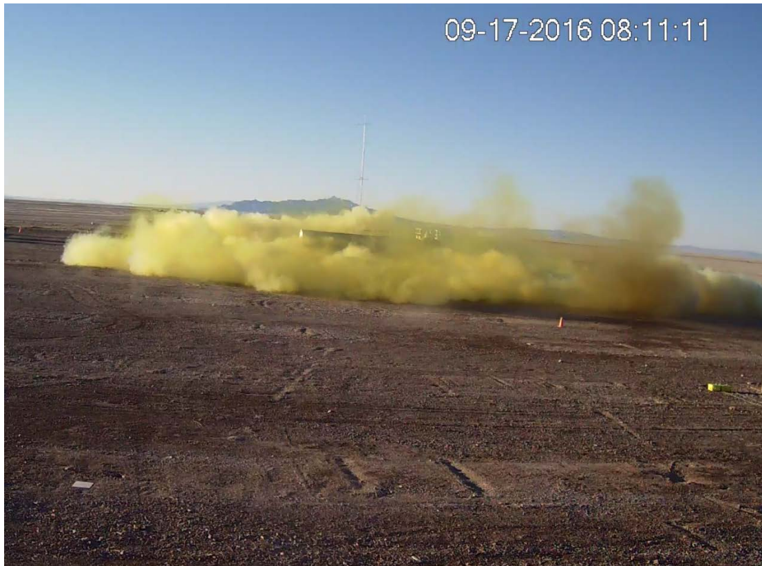
Figure 39. Release 9, 2016, 20 tons. Seconds after the release from 5 m elevation and 85 m downwind. Compare to the same time as seen from the UAV in Figure 38.
