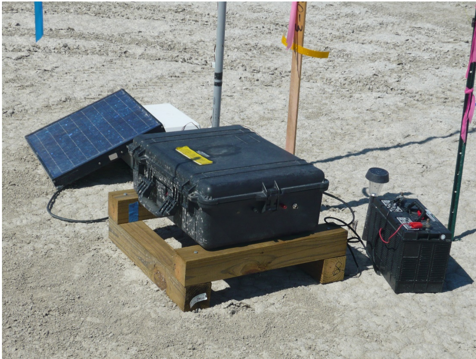
Figure 1. Typical JAZ ® deployment configuration.
