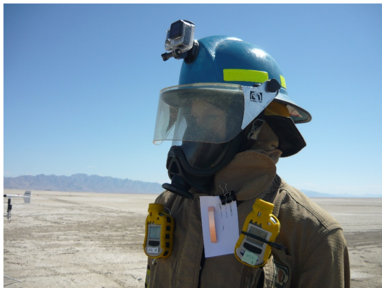
Figure 14. Release 9, 2016. A UVU and DPG ToxiRAE® detectors at the 100m mannequin upwind.
