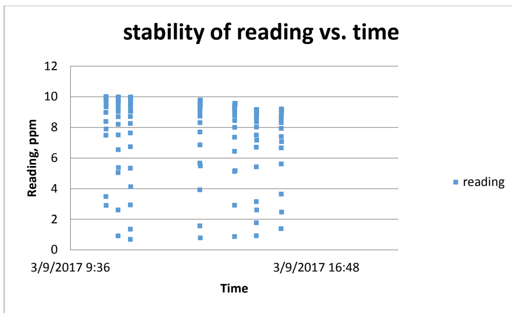
Figure 33. PID with an 11.7eV bulb with 80 hours of running time dropped only 10% in accuracy over a seven hour exposure.
