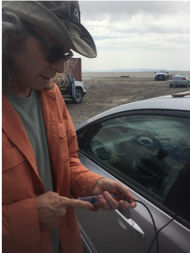
Figure 16. Dr. Delp from LBL injects a vehicle with SF 6 to determine the exfiltration rate (ACH).
