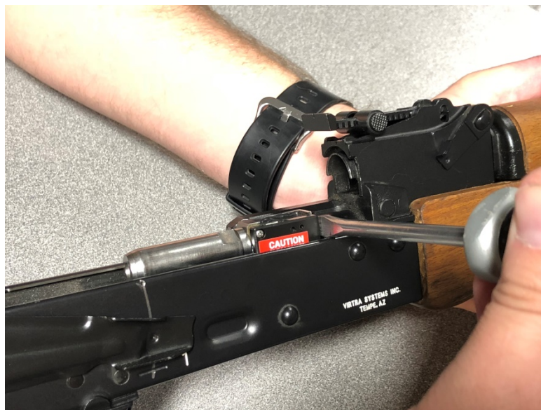
Figure 12: DO NOT PRY AT THIS LOCATION
