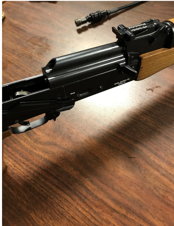
Figure 6: Bolt Carrier Fully Installed
