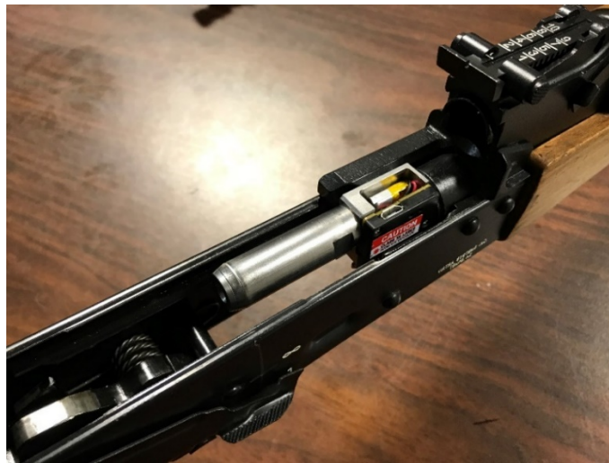
Figure 2: Charge Chamber Installation
