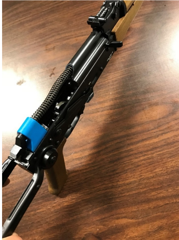
Figure 9: Recoil spring and Buffer Installation
