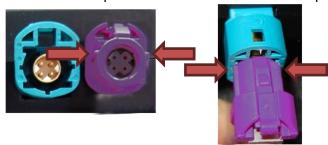
**Note:** The marked lug of the female 4pin HSD LVDS connector of the vehicle harness has to be cut off in some vehicles!
