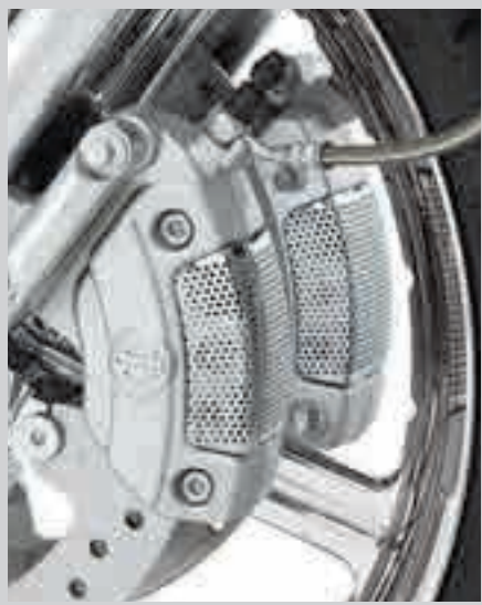
H. CHROME CALIPER SCREEN INSERT – FRONT SHOWN
