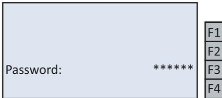
3. The terminal will prompt for the Supervisor password; once the password has been entered press the green **Enter** key.
