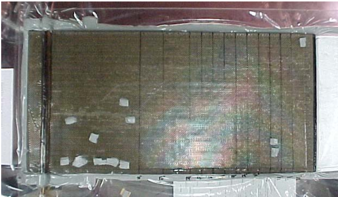
Figure 5.11 – 12.7 mm thick foam core preform with 12.7 mm stitch row spacing. The preform has been completely infiltrated.
