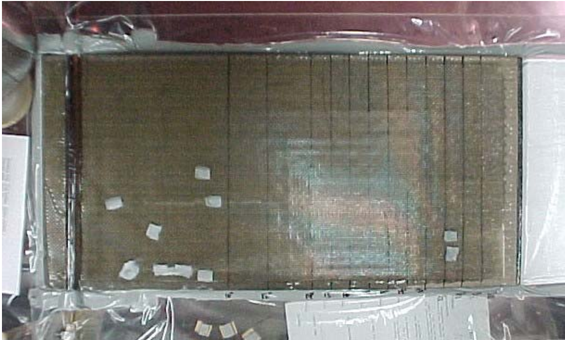
Figure 5.10 – 12.7 mm thick foam core preform with 12.7 mm stitch row spacing. Flow front is approximately 61.0 cm from injection edge.
