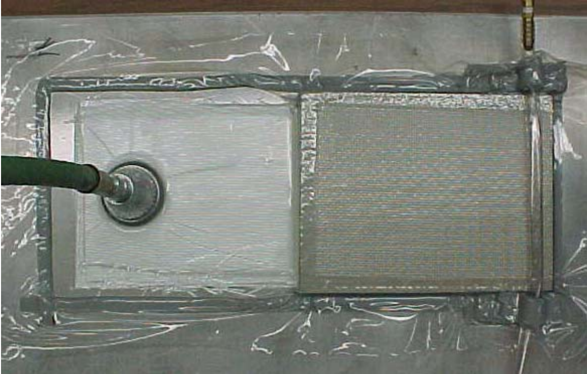
Figure 4.4 – VARTM processing set-up for a stitched foam core composite panel.
