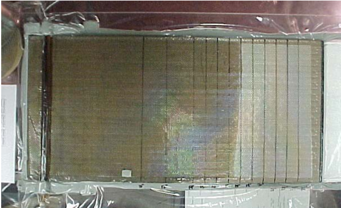
Figure 5.8 – 12.7 mm thick foam core preform with 12.7 mm stitch row spacing. Flow front is approximately 45.7 cm from injection edge.
