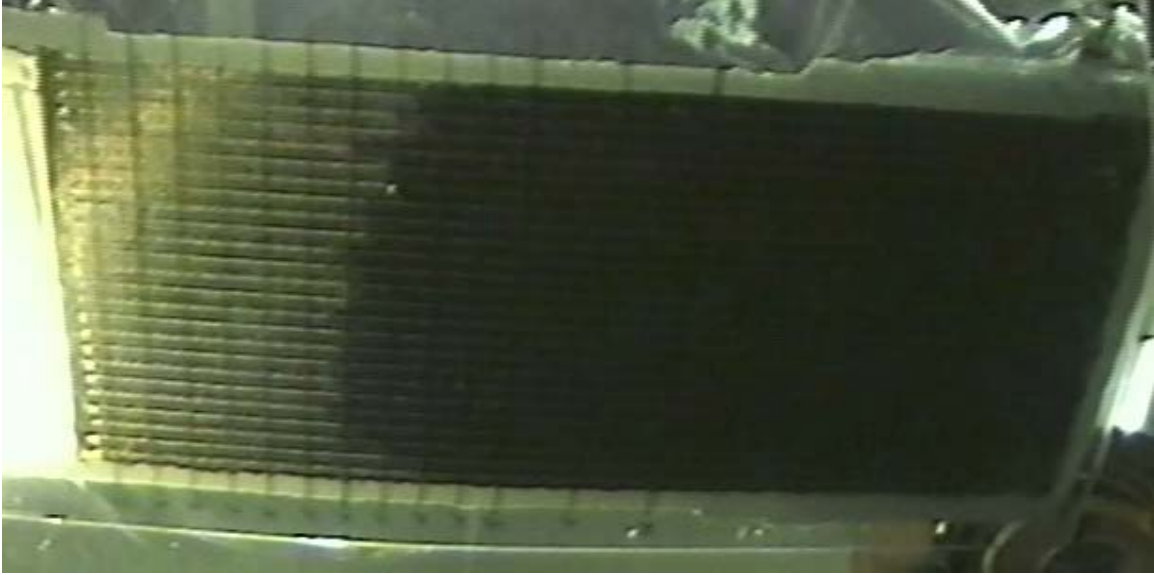
Figure 5.53 – Bottom surface of 25.4 mm thick foam core preform with 12.7 mm stitch row spacing. Flow front is approximately 45.7 cm from injection edge.
