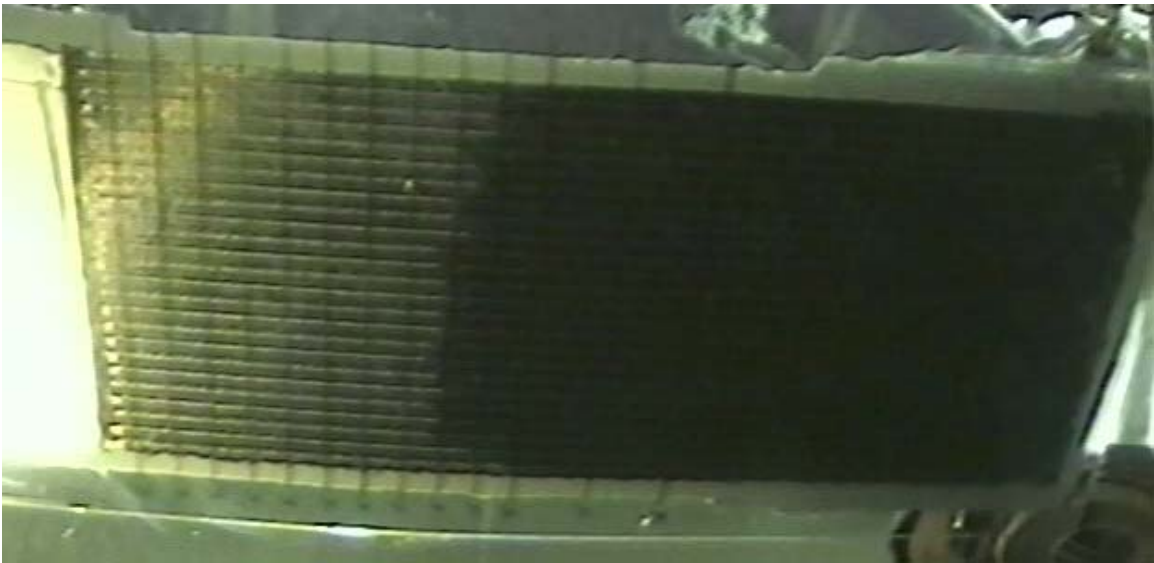
Figure 5.52 – Bottom surface of 25.4 mm thick foam core preform with 12.7 mm stitch row spacing. Flow front is approximately 40.6 cm from injection edge.
