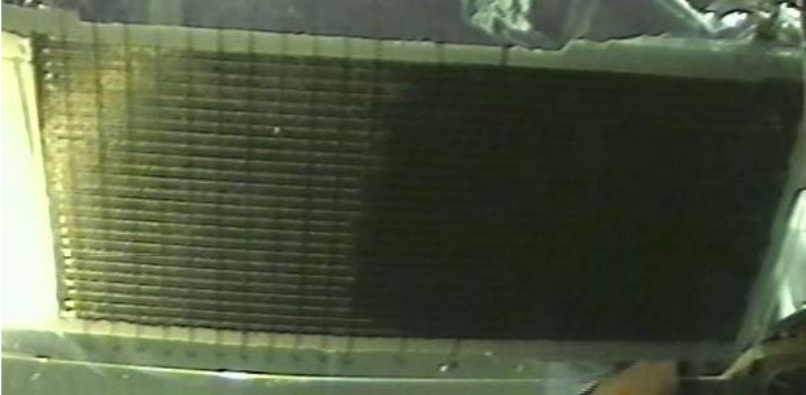
Figure 5.51 – Bottom surface of 25.4 mm thick foam core preform with 12.7 mm stitch row spacing. Flow front is approximately 35.6 cm from injection edge.
