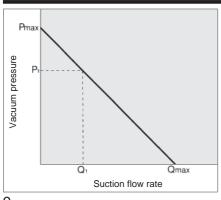
Flow rate characteristics are expressed in ejector vacuum pressure and suction flow. If suction flow changes, the vacuum pressure will also be changed. Normally this relationship is expressed in ejector standard operating pressure use. In the graph, Pmax is maximum vacuum pressure and Qmax is maximum suction flow. The values are specified according to catalogue use. Changes in vacuum pressure are expressed in the below order.
