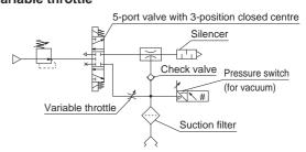
5-port valve with 3-position closed centre is used to control the vacuum generation and release. A check valve is installed to the vacuum port to prevent vacuum pressure from being reduced when the supply valve is OFF\*1. A pressure switch is installed in the vacuum circuit to detect pressure. A suction filter should be mounted to the position where the duct collected by release air can be flushed by released air.
