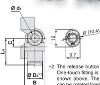
The release button of Ø 6 One-touch fitting is oval as shown above. The button can be rotated freely.
