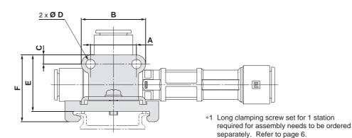
DIN rail mounting bracket (Brackets on both sides)\*2
