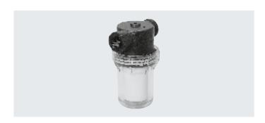
The vacuum filter is used to filter particles in the suction direction. The filter cartridge is located in a transparent bowl so that the degree of contamination of the filter cartridge can be determined. The filter cartridge can be replaced → page 7
