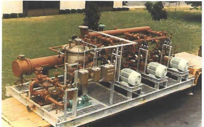
Liquid ring compressors for crude oil vacuum distillation tower.
