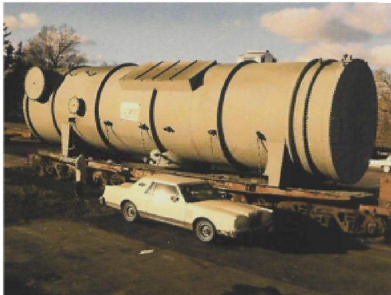
A 90,260 sq. ft. steam condenser for geothermal power plant in California.
