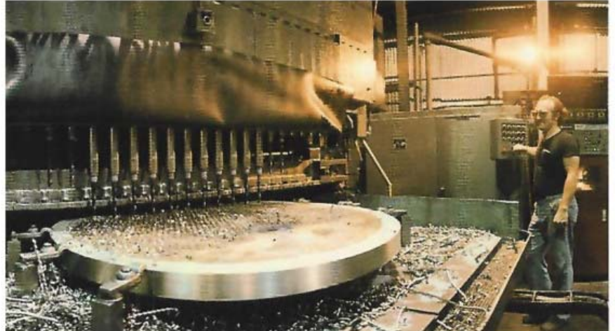
Computer-controlled 37 multi-spindle drill for tube sheets and support plates.
