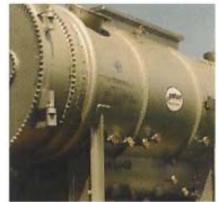
Steam surface condensers
