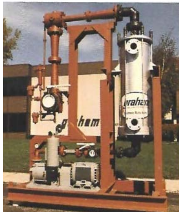
Combination system with graphite intercondenser for a pharmaceutical plant.
