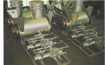
Condensers and air ejectors.
