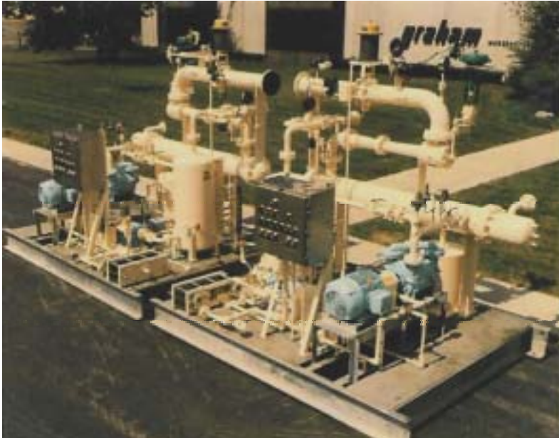
Two automated condenser exhauster packages with combination of ejectors and liquid ring vacuum pumps.
