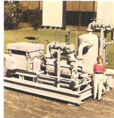
Large Condenser exhaust system.
