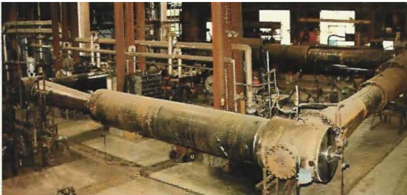
Testing first four stages of six stage ejector.
