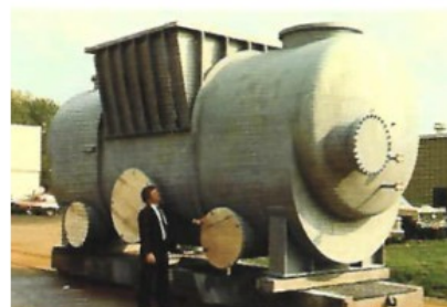
Direct contact horizontal condenser for 12.5 MW plant in Nevada
