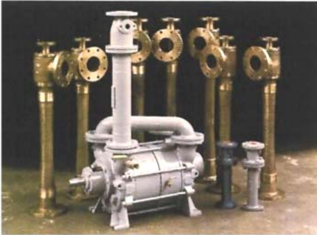
Bronze Ejectors and Liquid Ring Pump with air ejector for salt water deaerating service.
