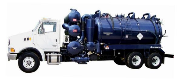
Cusco's Turbovac Series vacuum trucks are ideal for environmental remediation work – they'll handle heavy sludge, slurries and liquid waste materials without compromise. With cyclonic filtration technology, airflow ratings of 1,800 to 5,500 CFM, and powered with 28" Hg of vacuum, this system is the ideal solution for the most complex hazardous and non-hazardous waste removal, transportation, and remediation work.
