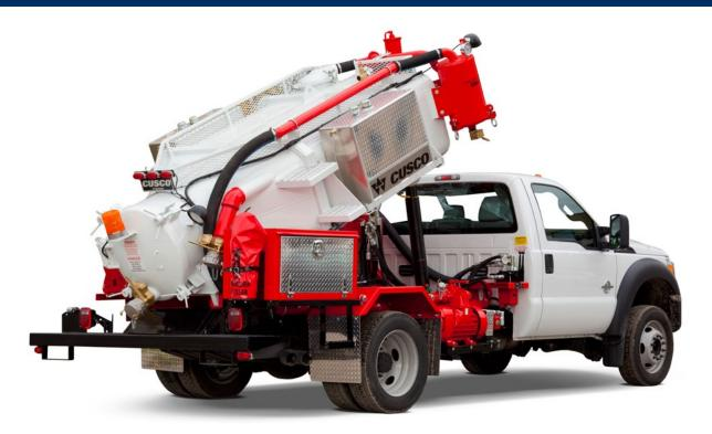
Cusco's Low Profile Series of vacuum trucks is ideal for working in low clearance levels, such as underground parking decks, or any low area where catch basins tend to be located. These trucks have a specially designed airlift system that enables the chassis to drop to a 77" clearance and return to its original ride height with the flick of a switch.
