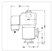
Dimensional drawing for the venting valve, electromagnetically actuated
