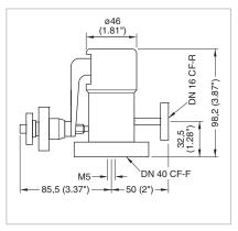
Dimensional drawing for the all-metal variable leak
