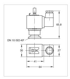
Power failure venting valves are open when de-energised and are used to automatically vent pumps, systems or vacuum vessels in the event of a power failure.
