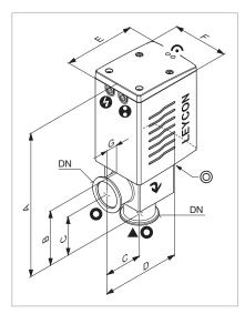
Dimensional drawing for the bellows-sealed right-angle valves
