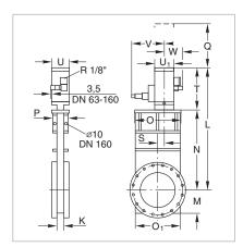
Dimensional drawing for the UHV gate valves CF electropneumatically ooperated
