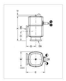
Dimensional drawing for the electropneumatically actuated right-angle valves
