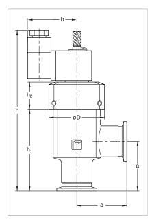
Dimensional drawing for the SECUVAC valves with ISO-KF small flanges
