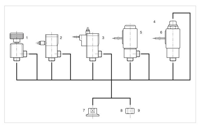
Oerlikon Leybold Vacuum small valves micro are available with any of four drive systems, two types of body and three adapters.
