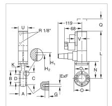
Dimensional drawing for the miniature UHV gate valves; electropneumatically operated, CF flange
