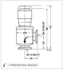
out isolation valve precisely defined quantities of gas may be admitted within a controllable period of time into evacuated vessels.
