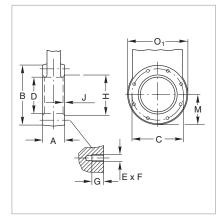
Connection dimensions for ISO-F flanges (UHV gate valves)
