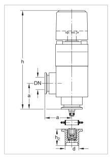
Dimensional drawing for the sealing valves
