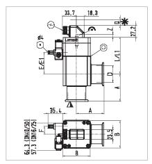
Dimensional drawing right-angle valves, with fitted pilot valve
