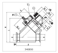
Dimensional drawing for the straight-through valves with fitted pilot valve (EP) without pilot valve (P) 1) pilot valve
