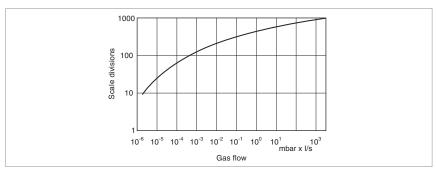
Variable leak characteristic for the variable leak valve with isolation valve
