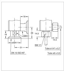
Connection dimensions for small valves micro
