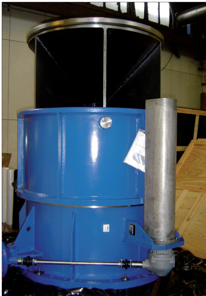
Picture 2: Transport position - vertical on the connection flange
