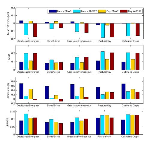
**Figure 7.** Four statistics results for SMAP L4 SM and AMSR2 L3 SM monthly and daily data with different vegetation cover types.
