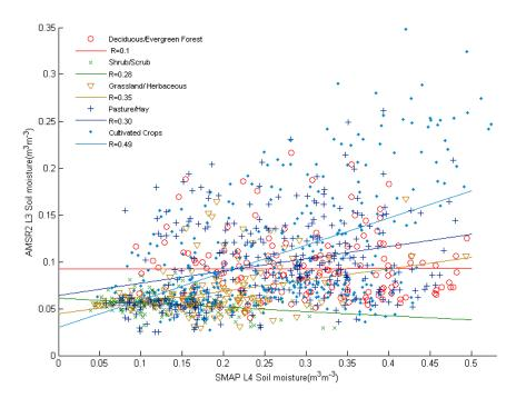
Figure 5. Comparison Soil moisture in different land covers between SMAP L4 and AMSR2 L3 data.
