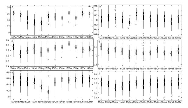
**Figure 10.** Temporal evolution of correlation between SMAP L4 (**a**,**c**,**e**) or AMSR2 L3 (**b**,**d**,**f**) daily average data and in situ soil moisture data in the western (**a**,**b**), central (**c**,**d**), and eastern (**e**,**f**) regions of U.S.
