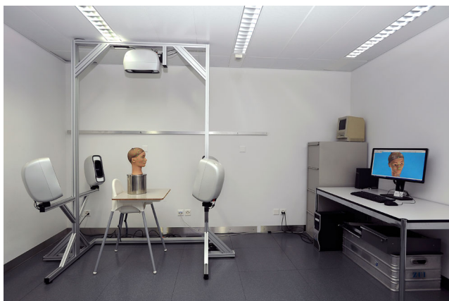
Fig. 2 Set-up of the 3D photosystem and mannequin head labelled with 52 landmarks covering all craniofacial regions
