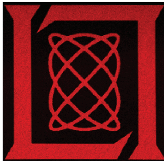
Figure 16. Raman image of the in-plane E_{2g} mode of tungsten disulfide grown by vapor phase epitaxy and patterned at a large-scale (figure is 400 \mu\text{m} on a side) using optical lithography and plasma etching.
