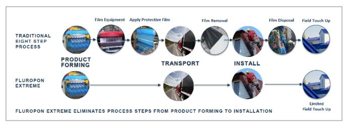
By eliminating steps in the production process, Fluropon Extreme coating delivers total cost savings. Metal coaters do not have to apply a protective film to protect the finish during transport, which eliminates wrapping, removal and disposal of the film. For coaters that didn't use film, there is no need for coating touch-up of scratches that occurred during transit.
