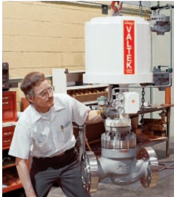
(Left) Despite an oxygen fire, this 4-inch high pressure Mark One properly fail-closed; thus, avoiding a catastrophe at an oxygen plant. Although the excessive heat eventually rendered the actuator inoperable, the flow direction (flow over the plug) allowed the valve to remain closed, preventing the fire to migrate past the seat. (Right) The same valve following servicing demonstrates Flowserve's expert repair services.
