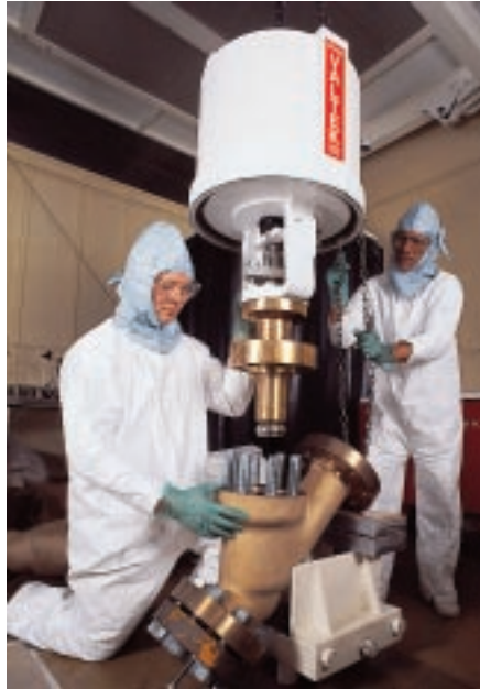
(Left) One of two massive "Titan" valves and hydraulic skids used in high temperature sodium service at a California sodium pump test facility.
